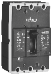
XF2 Frame : I cu /I cs = 25/25, 36/18, 36/27, 36/36, 50/25, 50/50 kA
